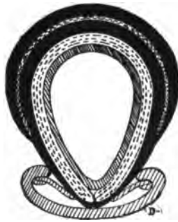
FIG. 108.—The "Grappler" Tire. Instead of endless wires, this tire carries projecting flanges of metal strips at either side of the base, which press against the inner overlapping sides of the channel rim, affording a secure attachment.
